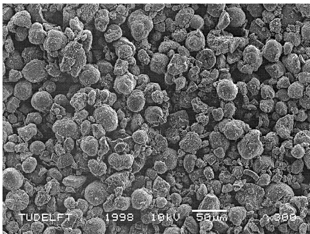
Fig. 5. Surface of \text{LiMn}_2\text{O}_4 + carbon black + PVDF coating on copper foil.
